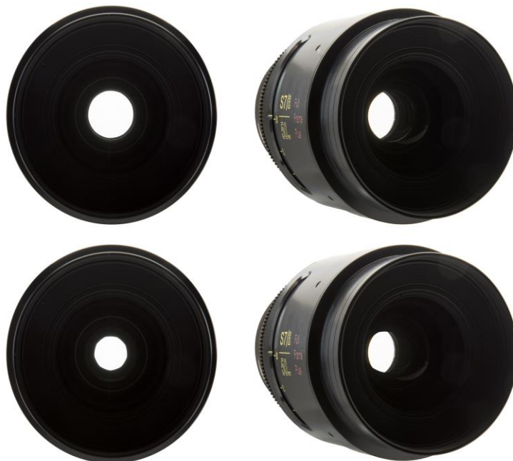
Figure 1: Optical vignetting on an example lens, with the iris set to f/1.4 (top row) and f/2 (bottom row). When viewed straight on (left column), the light collection area is defined purely by the lens's iris. From an angle, the light collection area is defined by the extent of the front and rear elements (at f/1.4 , top right), or by the front element, rear element, and iris (at f/2 , bottom right).
