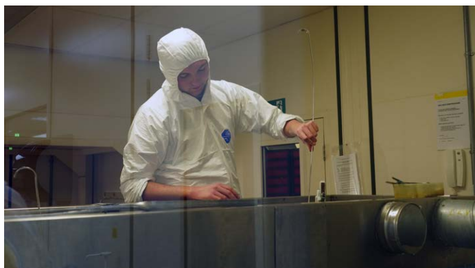
Clean the optical elements before coating.
