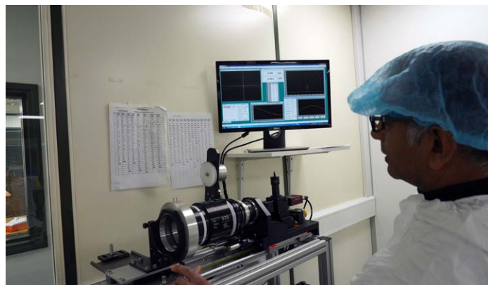
These days (2020) he now confirms accurate focus with an MTF display.
