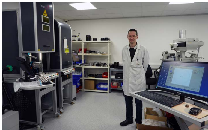
Each mark is lined and identified. The lens then goes to the engraving room. Laser engravers are seen above at left. CNC engravers are at right.
