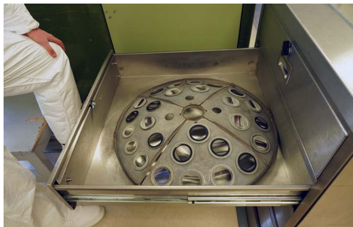
Load the optical elements onto carrier.
