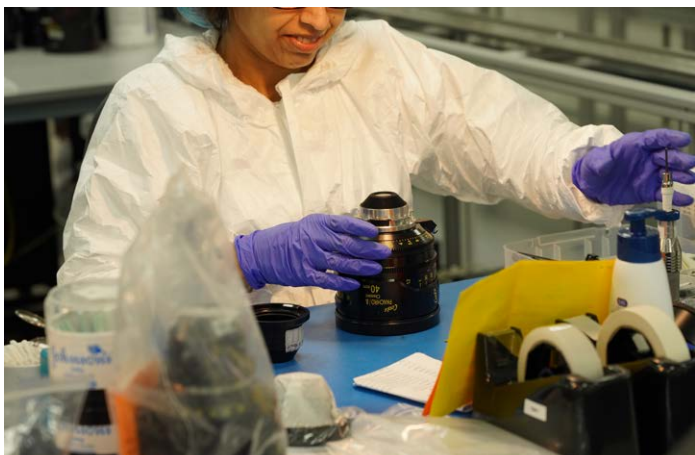
Securing the /i technology electronics into a Panchro/i Classic 40mm.
