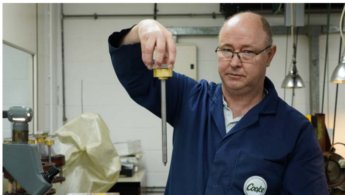
Edging ensures the element fits into its mechanical supports within the barrel. Paul Utting demonstrates: once cool, the pitch is like glue.
