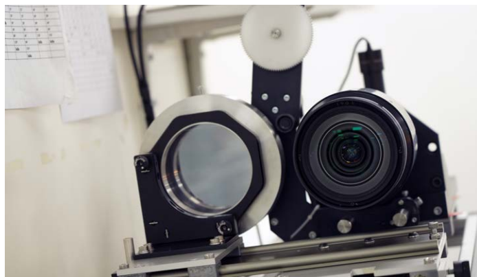
Infinity is established with a supplemental mirror.
