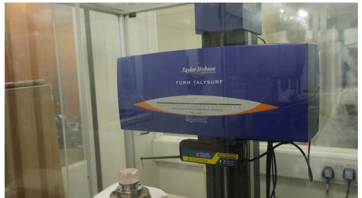
The Form Talysurf measures aspheric polishing inconsistencies. The original Talysurf 1 by Taylor & Hobson Talysurf was introduced in 1941 to accurately measure surface texture.
