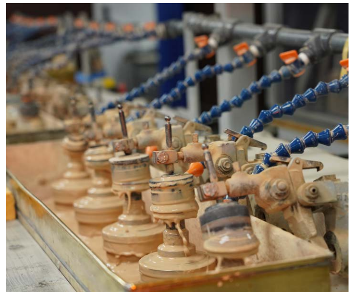
The polishing compound is an abrasive slurry of Cerium Oxide.
