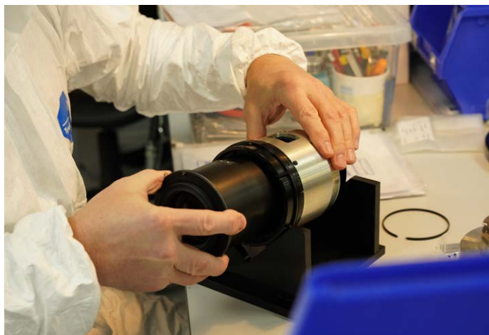
Inners (sub assemblies) slide into outers.
