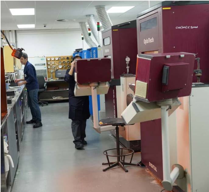
OptoTech CNC lens grinding machines.
