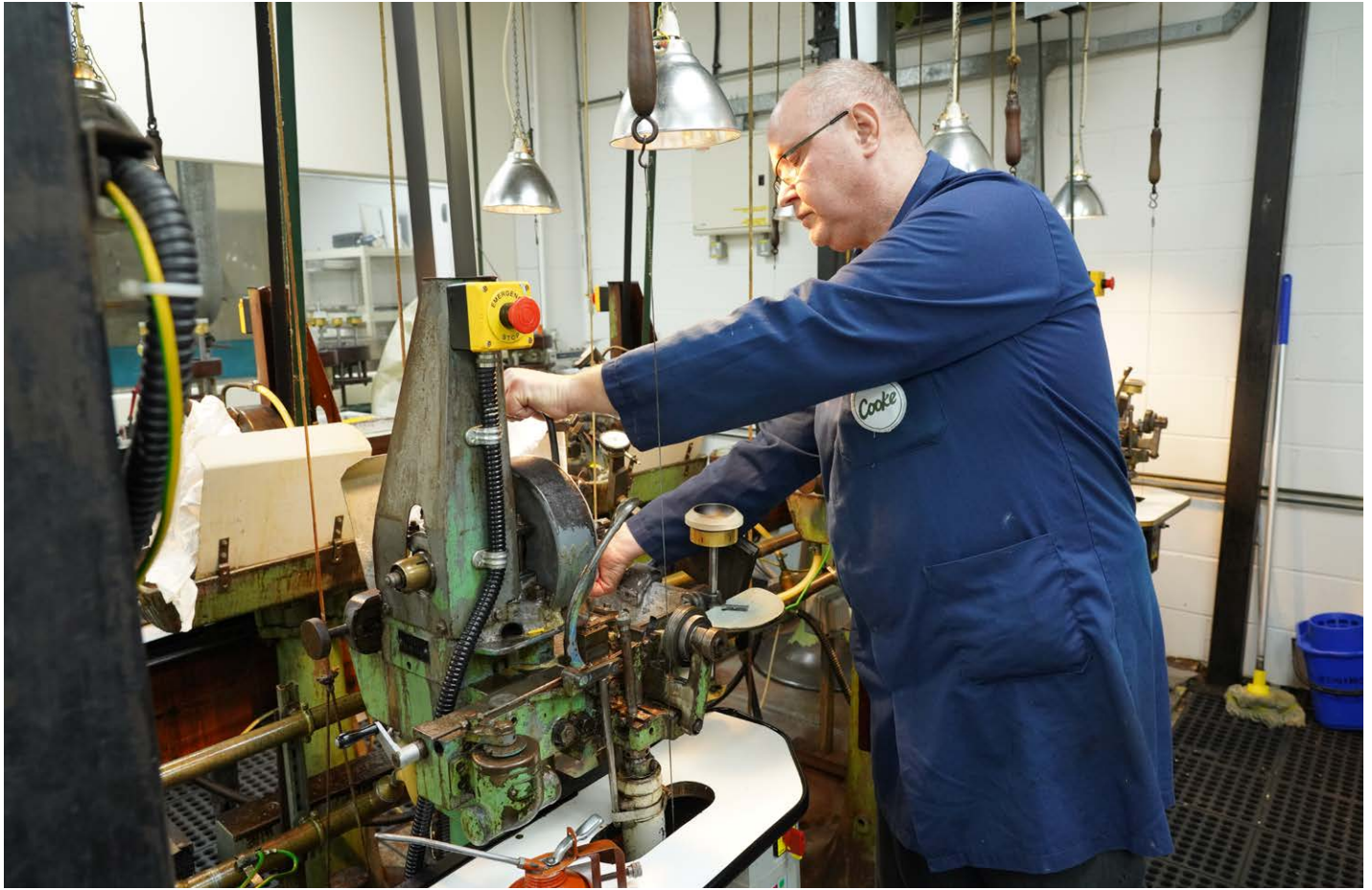
Vintage machines in the hands of a master craftsman like Paul Utting can produce accurate results to tolerances of less than 5 microns.
