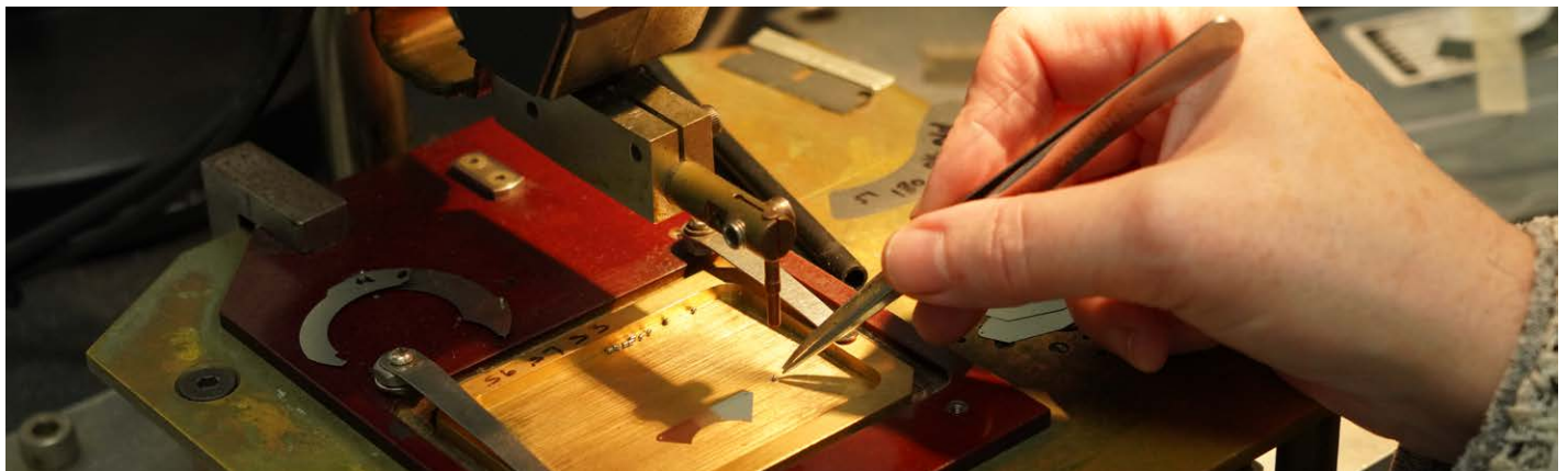
Iris leaf pins are welded into position.
