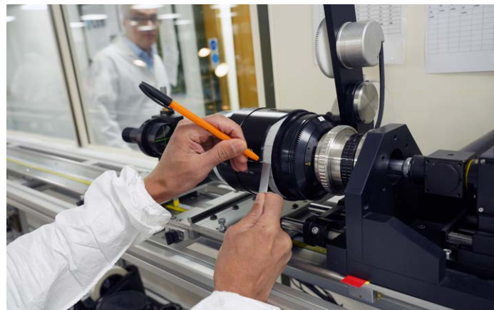
Each mark is lined and identified. The lens then goes to the engraving room. Laser engravers are seen above at left. CNC engravers are at right.
